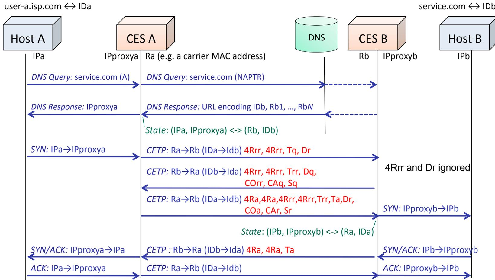
4Rrr=RLOC Reliable reply, 4Ra=RLOC Ack, Tq=Timeout query, Trr=Timeout reliable reply, Ta=Timeout ack, Dr=Domain reply, COrr=Cookie reliable reply, COa=Cookie Ack, CAq=CA Address query, CAr=CA Address reply, Sq=Signature query, Sr=Signature reply
