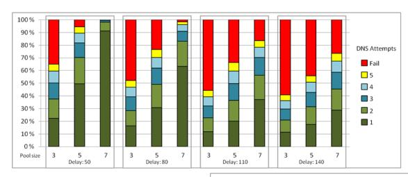
Impact of delay and pool size with a fixed load of 60 new connections per second
