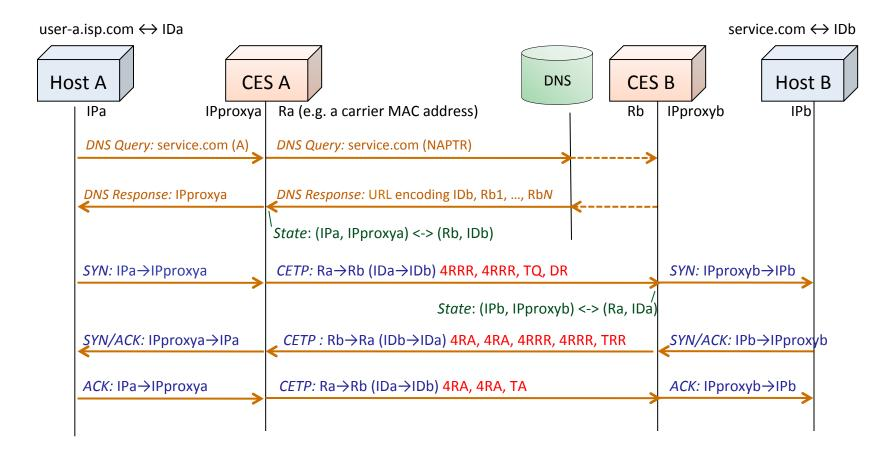
4RRR=RLOC Reliable reply, 4RA=RLOC Ack, TQ=Timeout query, TRR=Timeout reliable reply, TA=Timeout ack, DR=Domain reply
