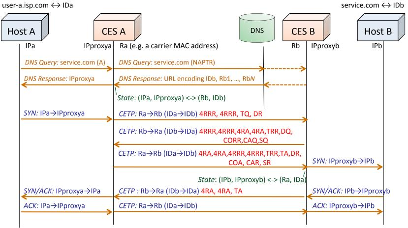
4RRR=RLOC Reliable reply, 4RA=RLOC Ack, TQ=Timeout query, TRR=Timeout reliable reply, TA=Timeout ack, DR=Domain reply, CORR=Cookie reliable reply, COA=Cookie Ack, SQ=Signature query, SR=Signature reply
