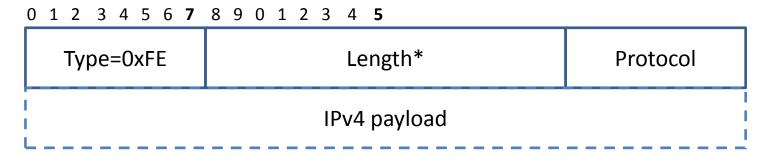
This resembles RFC-2004: Minimal Encapsulation within IP and assumes that the core transport takes place over IPv4. Unlike in RFC-2004, not even the destination IP address is preserved because it must be mapped by the receiving CES based on target ID.
